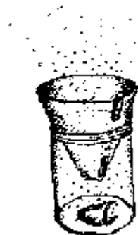
Fruit fly trap made from a jar and a paper funnel. Bait with cider vinegar or slice of banana.
